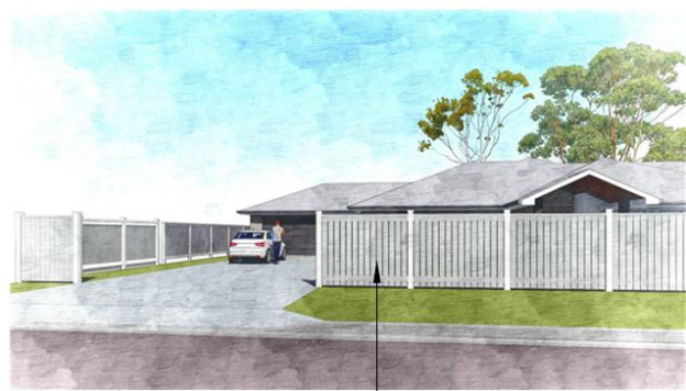
Inappropriate fence design does not enable casual surveillance of the street
