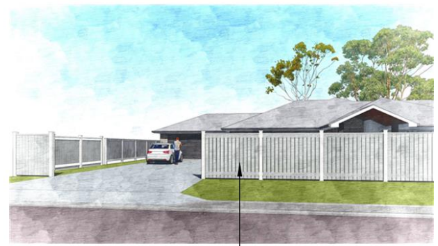
Inappropriate fence design does not enable casual surveillance of the street
